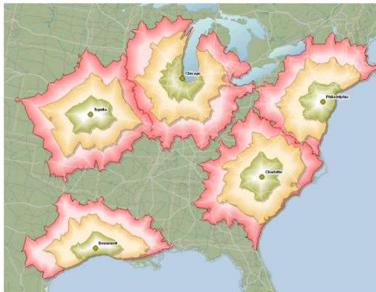
Fig. 4. Two, four and six hour service areas around five cities (from http://desktop.arcgis.com/en/arcmap/latest/extensions/network-analyst/service-area.htm ).
